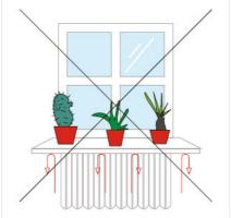
If there is a heater underneath the window, there should not be a flower shelf above it without a sufficient air gap between the shelf and the wall. The flow of warm air along the window glass is also obstructed by excessively wide window ledges as well as drawn curtains and plants placed on the window ledge.
